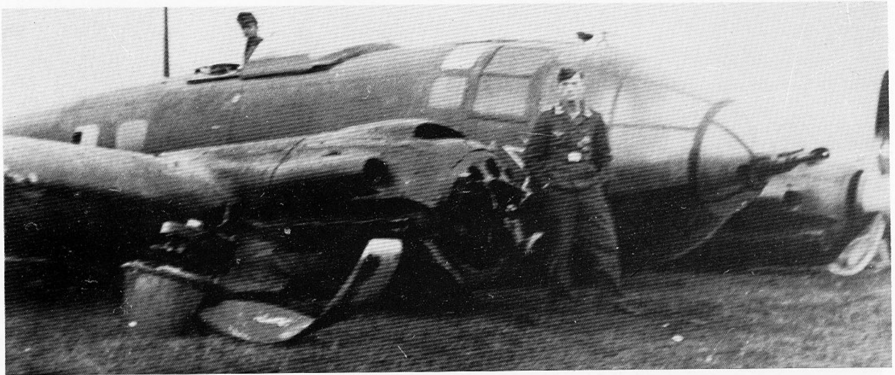
Crash landing of an He 111 H-6 armed with an MG FF in the nose gunner's station.
