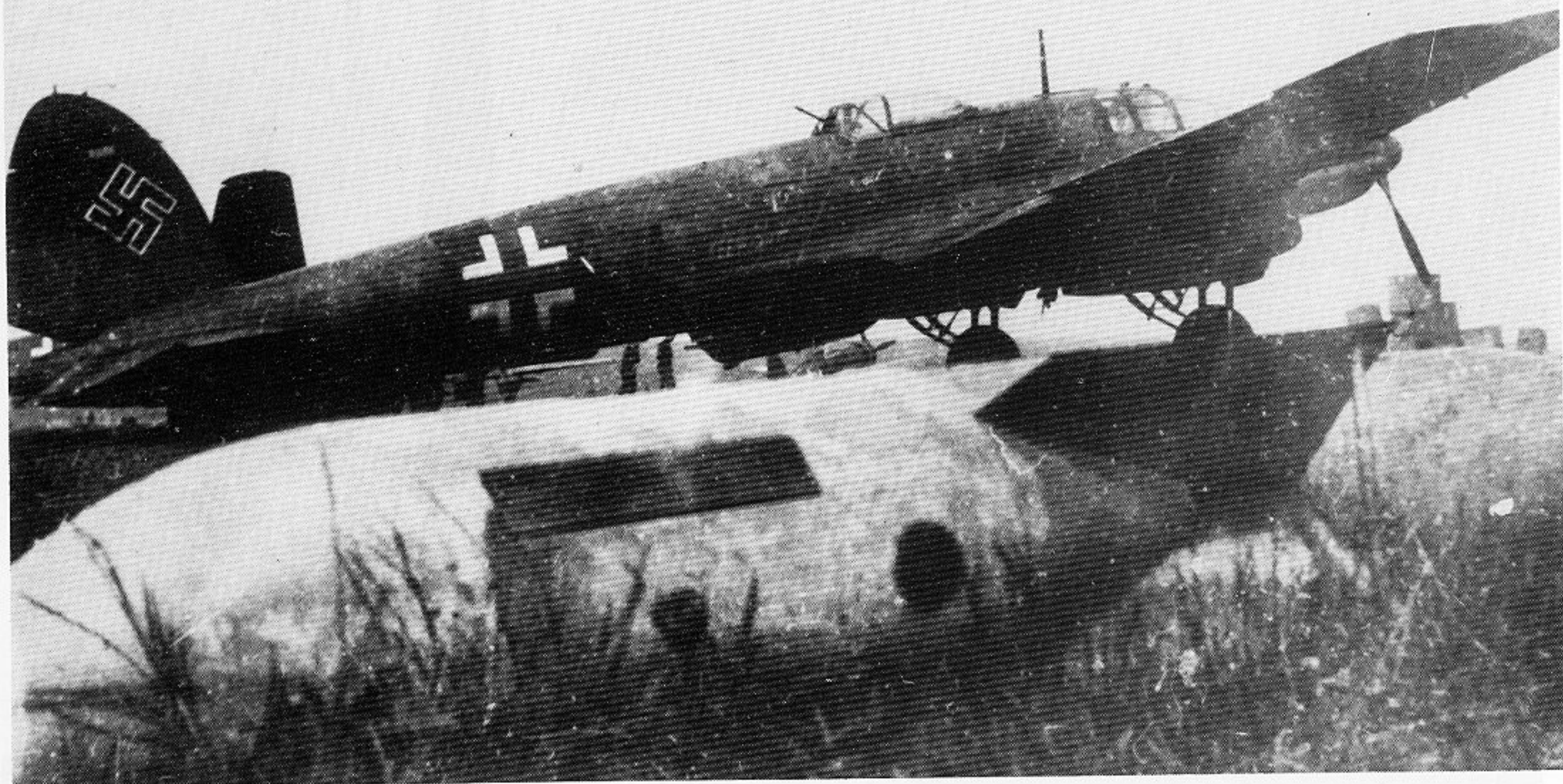
During the development of the He 111 H it wasn't just the defensive armament which was constantly being strengthened,; passive armor (around the dorsal gun position) was also improved.
