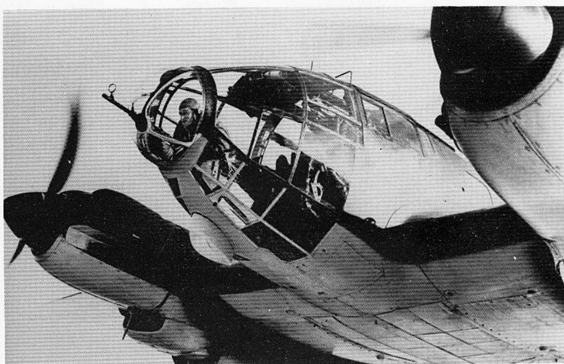
Close-up of the He 111 H-1 canopy with an MG 15 in the nose gunner's position. Bomb bay doors are clearly visible.
