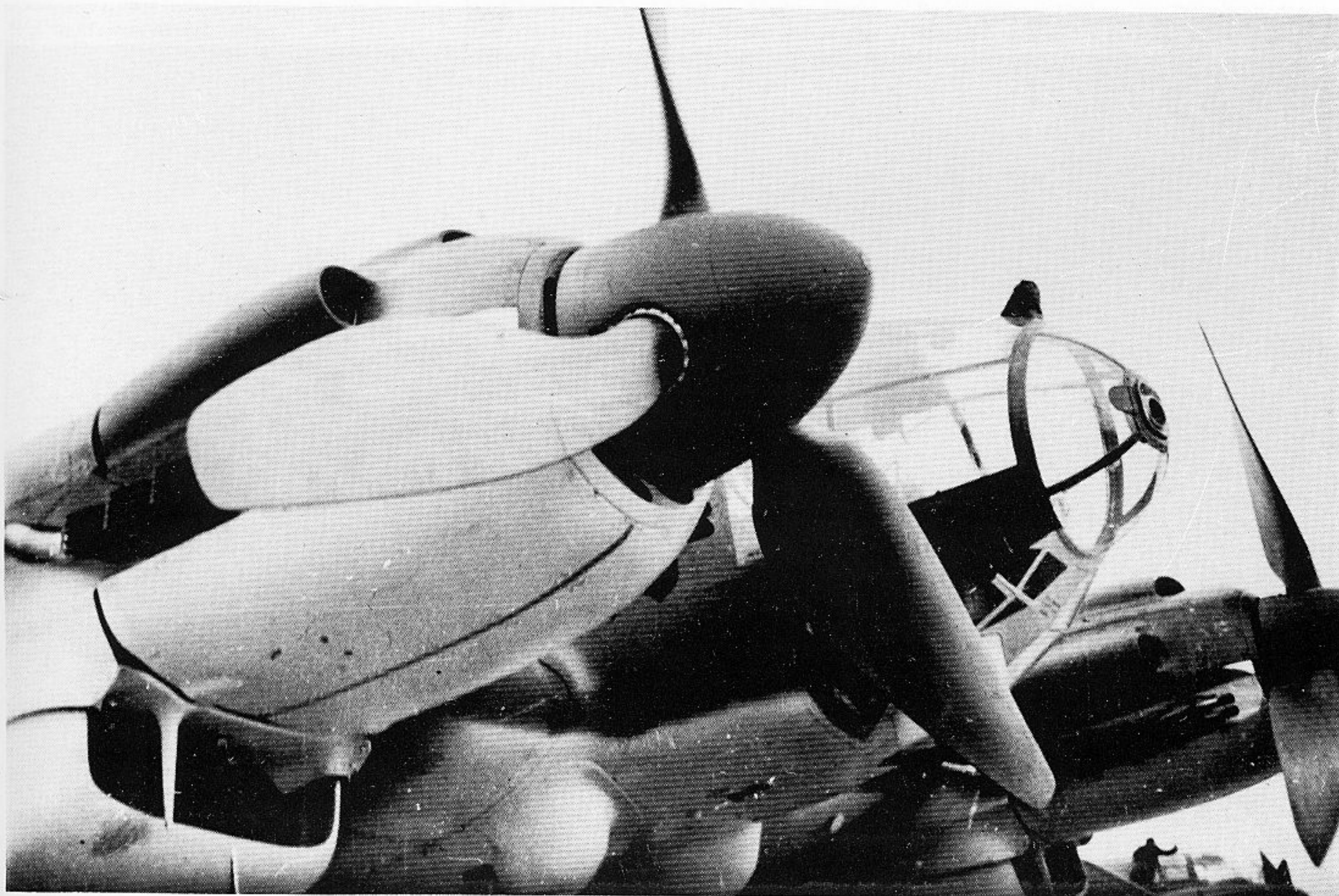
He 111 H-4 test flight operations at the Oranienburg factory. Notice the openings in the nose canopy for two MG 15s.
