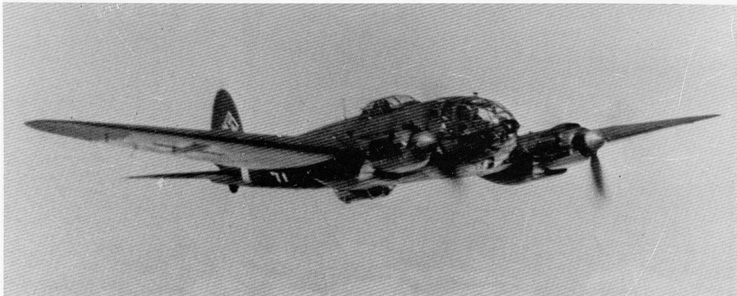
Above and below: This He 111 H-11 was fitted with an FuG 101 precision altimeter and a "Kutonase" for low-level attacks.
