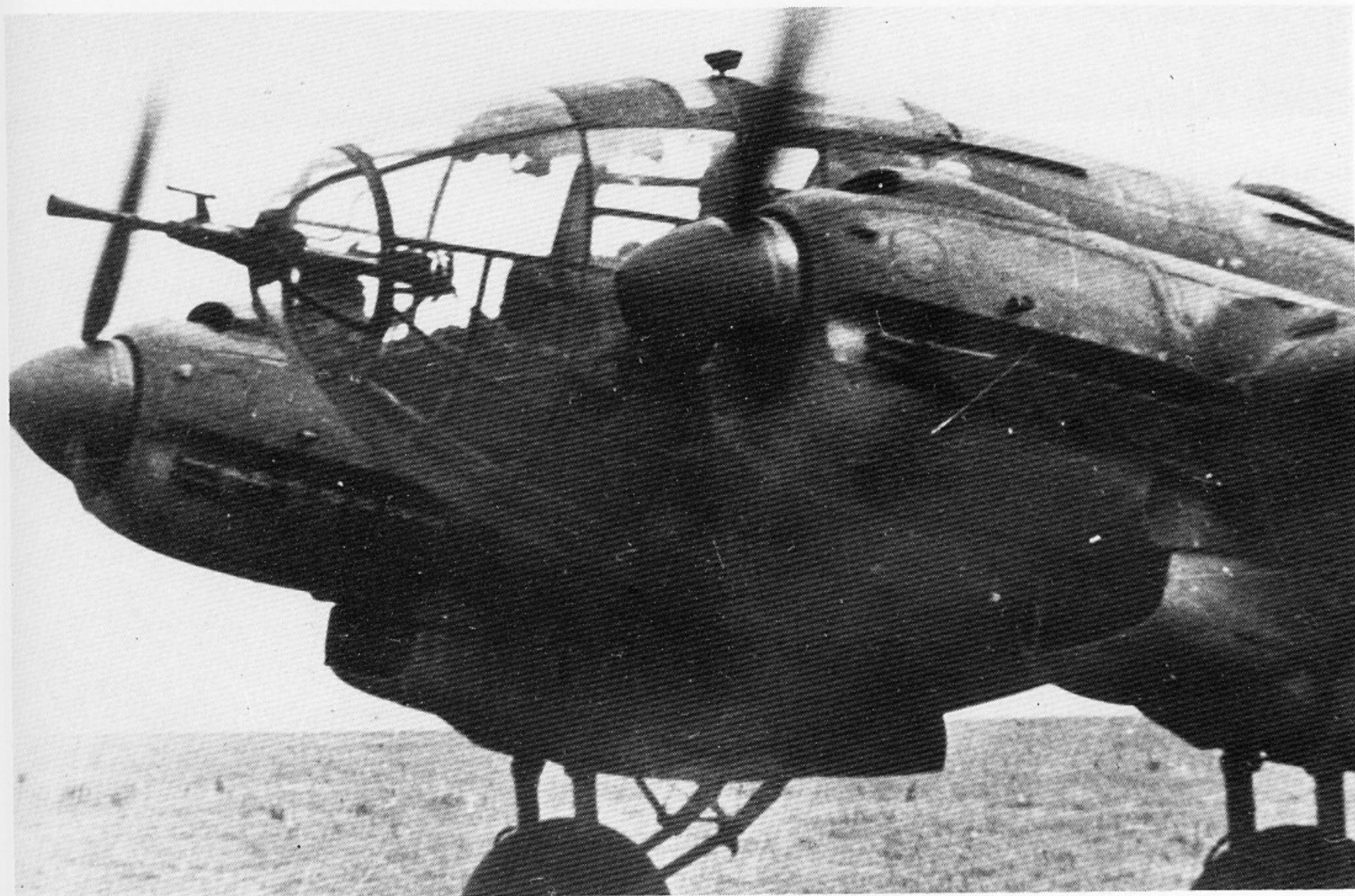
The He 111 H-18 was designed exclusively for the night bomber role; having 2 x 4 ESAC bomb racks it was incapable of carrying the heavier bombs.
