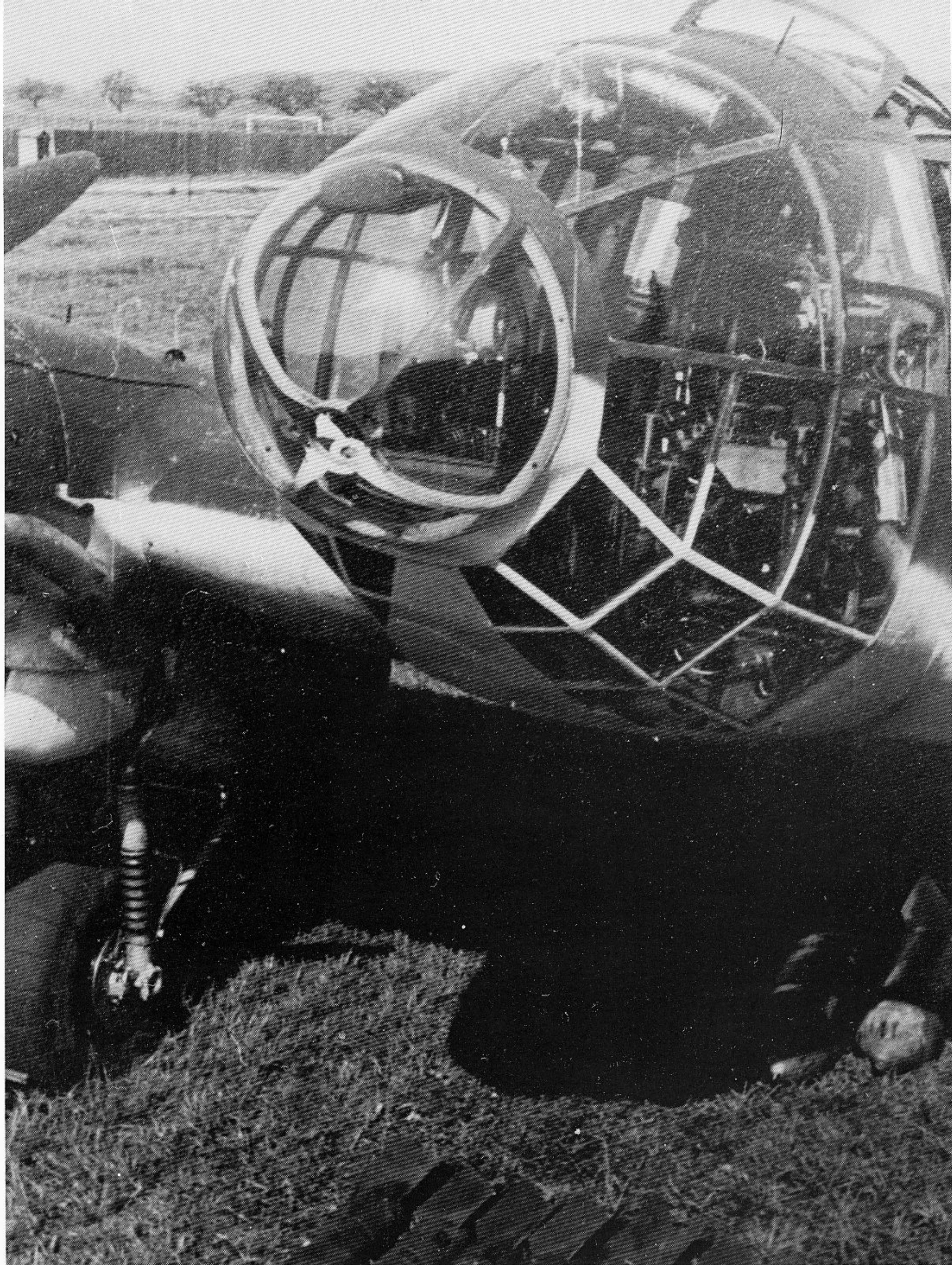
An He 111 H-3 ready for the next mission. Notice the adjustable window above the pilot's seat.
